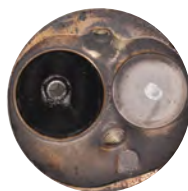
Cylinder head after one P.i. treatment.
